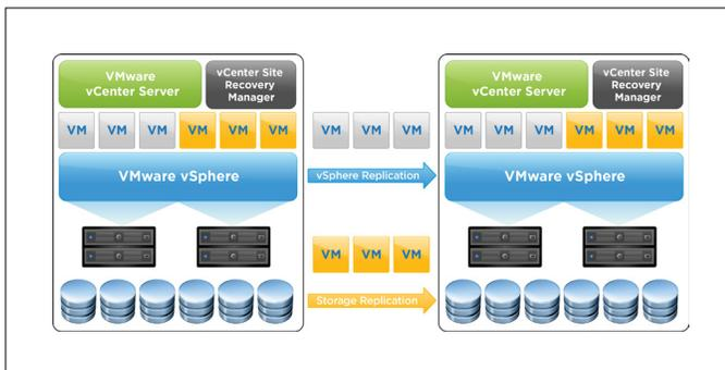
vCenter Site Recovery Manager automates the failover and migration of virtual machines to a secondary site. vCenter Site Recovery Manager relies on either vSphere Replication or a storage-based replication product to replicate virtual machines to the recovery site.
